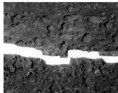
Figure 6. Inside surface at the failure origin of a 20-inch pipeline.
