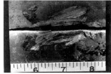
Figure 3. A 3-1/2 inch long gouge found near the midpoint of the rupture shown in Figure 2.
