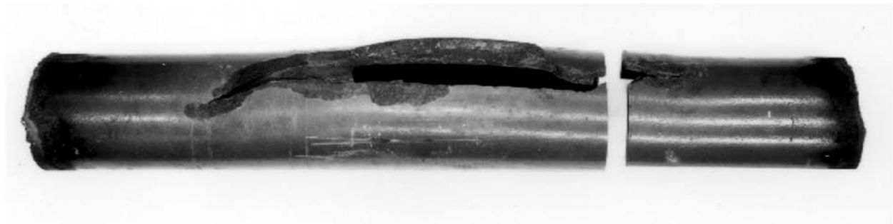
Figure 11. Hydrostatic test rupture of seamless 6-5/8 inch O.D. pipeline showing thin tongue of metal protruding from around a pipe lamination.
