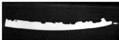
Figure 7. Cross section taken adjacent to the fracture shown in Figure 6. The arrow identifies the fracture surface in the pipeline.
